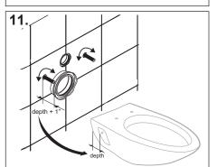
Use slotted end of thread bolt to adjust in or out. Do not damage the thread.
