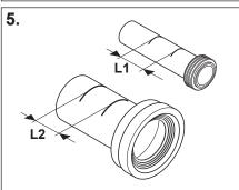
Measure distance between both lines on pipes. Take measured distance, deduct from bald end of pipe and cut.
