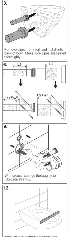
Install with mounting hardware and ensure toilet bowl is level.
