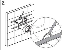
With a ruler, against finished wall, on top of pipe, mark as shown.
